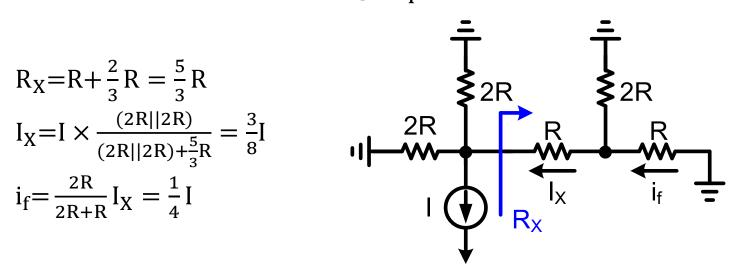
• With similar analysis, it can be shown that the current through  $b_4 \& R_f$  is I/8. Therefore,
